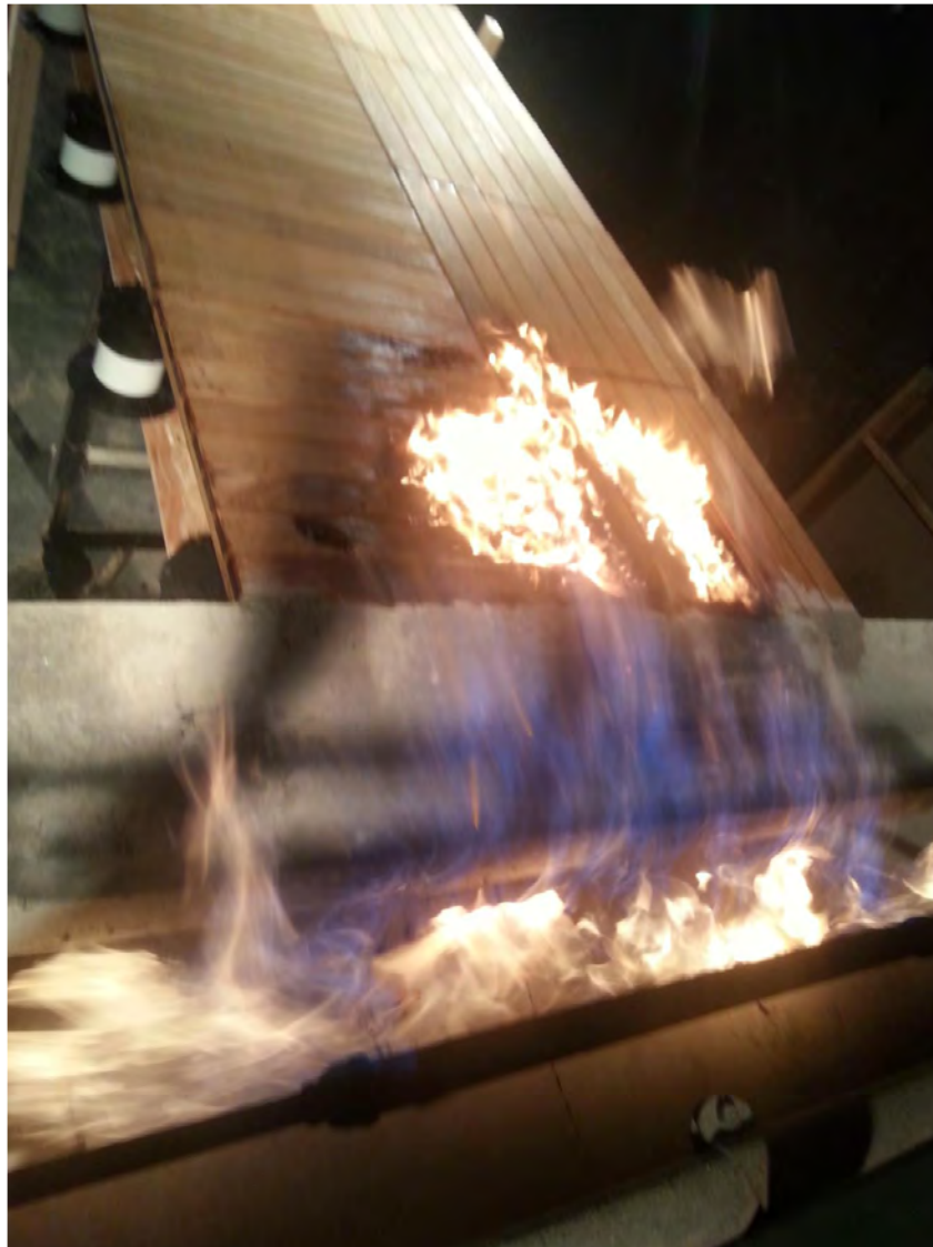
Photograph 2: Ipe Wood Tile Deck at Maximum Flame Spread
