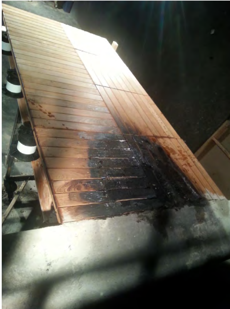
Photograph 3: Ipe Wood Tile Deck After Test Completion
